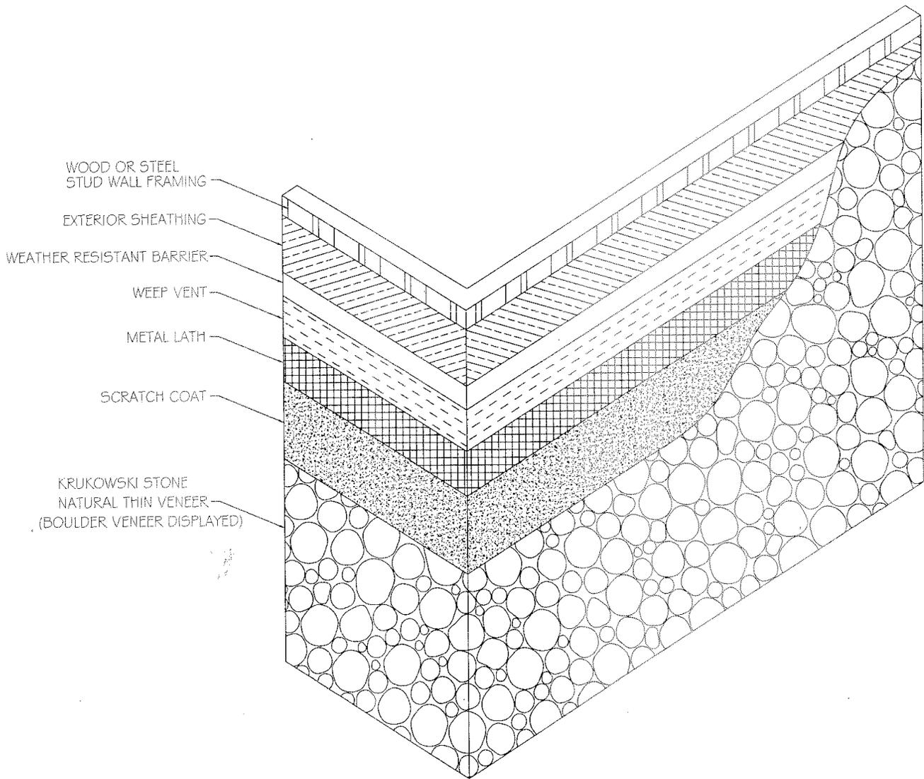
TYPICAL WOOD OR STEEL EXTERIOR STUD WALL
