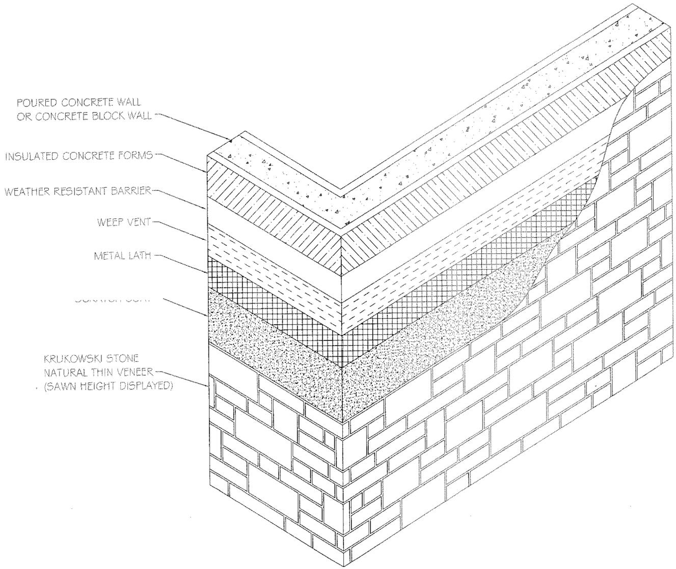
TYPICAL INSULATED CONCRETE FORM WALL
